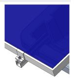
Fix 4 pcs 140mm mini rails on the side of plastic trays by 8pcs 6.3\*25 screw or 4 pcs 200mm mini rails by M8\*30 bolt set, then fasten the aluminum end clamps to install the solar panels.
