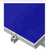
Fix 4 pcs 140mm mini rails on the side of plastic trays by 8pcs 6.3\*25 stepping screw or M8\*30 bolt set, then fasten the aluminum end clamps to install the solar panels.
