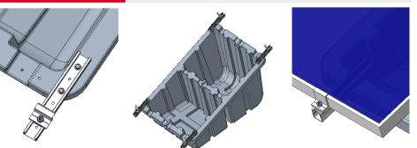
Fix 4 pcs 140mm mini rails on the side of plastic trays by 8pcs 6.3\*25 stepping screw or M8\*30 bolt set, then fasten the aluminum end clamps to install the solar panels.
