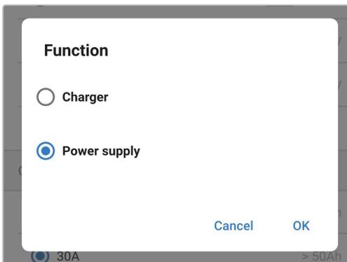
6. After a short delay the BULK, ABS, FLOAT and STORAGE LEDs will be illuminated to indicate the charger function has changed to Power supply mode.
