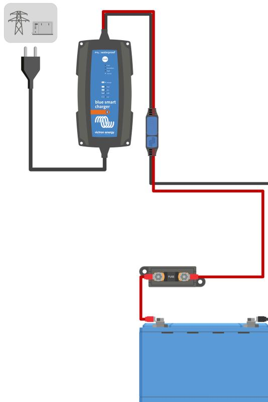
3. Connect the **Blue Smart IP65 Charger** AC power cable to a mains power outlet; after a short delay the TEST LED will begin to blink, until the charger determines if the battery will successfully accept charge (for up to 2 minutes).
