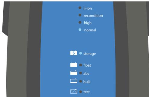
2. Press (and release) the **MODE** button on the **Blue Smart IP65 Charger** to cycle through and select the most appropriate integrated charge mode (Normal, Normal + Recondition, High, High + Recondition or Li-ion).
