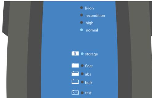
2. Depress and hold down the MODE button on the **Blue Smart IP65 Charger** for 10 seconds.
