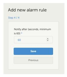
Note that the time set is the amount of time the high or low condition is active before an alarm is generated. It can then take an additional amount of time (up to 15 minutes) before that alarm is sent to VRM and an email notification is sent.
