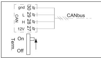
Fig. 19 Termination CAN-BUS
