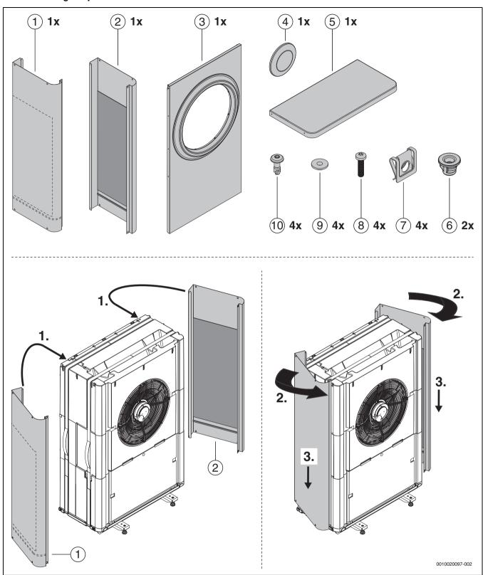
Fig. 21 Installing side panels and cover
