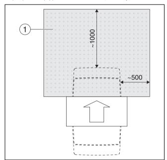
Fig. 11 Danger! Ice formation in front of the heat pump with sound hood (accessory)
