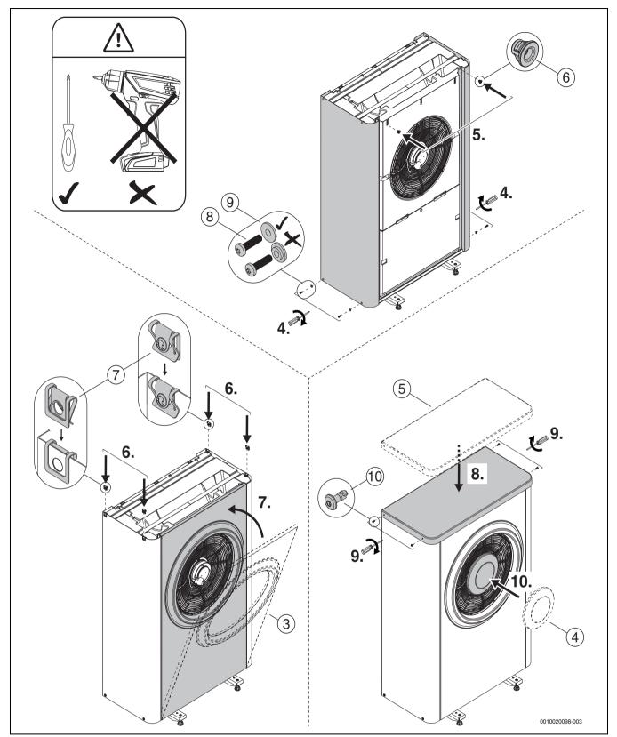
Fig. 22 Installing side panels and cover
