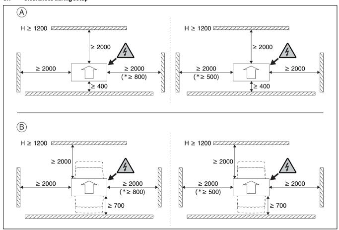
Fig. 8 Clearances during setup
