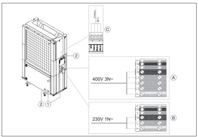
Fig. 20 Cable conduits and control device
