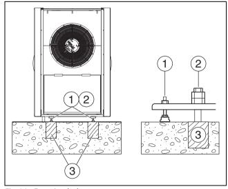
Fig. 14 Fastening the heat pump
