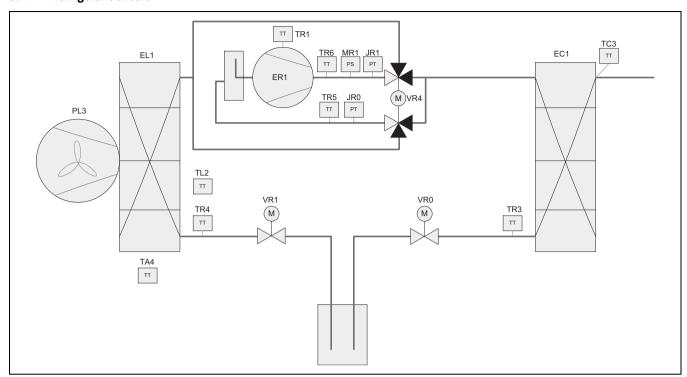
Fig. 24 Refrigerant circuit
