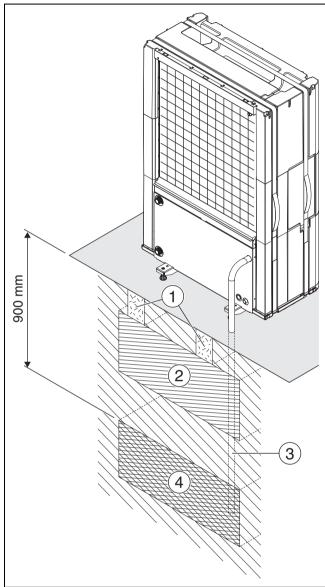
Fig. 12 Condensate pipe in gravel bed
