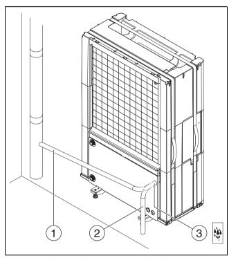
Fig. 17 Condensate tube connections, valid for all sizes
