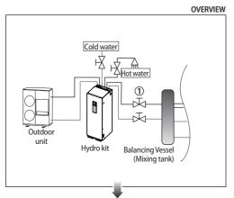
Sanitary warm water Tank Diagram(Field Scope)
