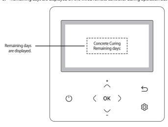
\* If an error is displayed, concrete curing function does not work.
