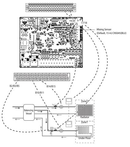
You can operate the 2-zone control using a mixing value, water-out temperature sensors, and built-in or external room temperature sensors installed in a wired remote controller.
