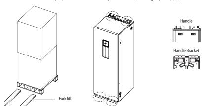
▶ Remove the handle bracket, wooden pallet the unit is in final installation location
