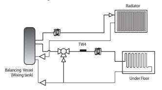
When two different zones are used with different temperature, adjust the temperature of discharge water to high temperature water and control the amount of bypass to provide low temperature water by applying the mixing valve and temperature sensor of the mixing valve (TW4).
