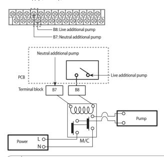
• The maximum allowable current that this terminal block can supply for the additional water pump is 0.1 A.
