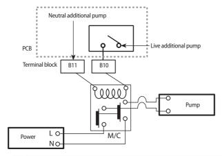
• The maximum allowable current that this terminal block can supply for the additional water pump is 50mA.
