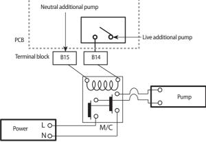
The maximum allowable current that this terminal block can supply for the additional water pump is 50mA.
