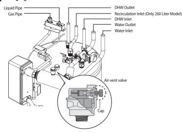
After installation is completed the following procedures shall be used to charge water into the hydro unit.
