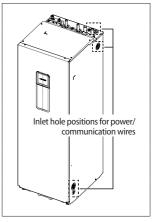
\* When you use inlet hole through the cabinet top positions for power/communication wires, please fix the wire by using mount tie of the cabinet right.
