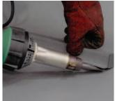
EJObar can be easily hot welded to make a very strong fix
