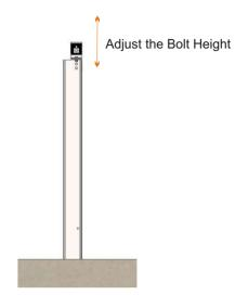
Step 2: Install and adjust the Top Cap
