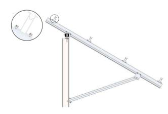
Step 4: Install the B-Rail by Rail Clamp
