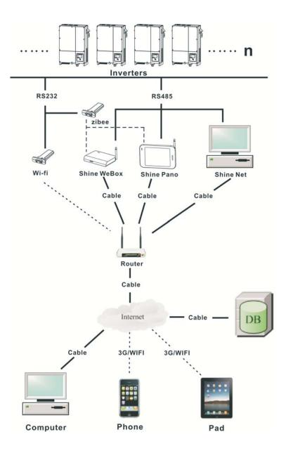
**i** Information When three phase inverter and single-phase inverter shared a RS485 communication line, the total length of which does not exceed 1km.
