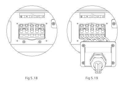
3) Fasten the protection shell onto the bottom of the inverter, make sure the four screws are tightened, the completed appearance is like the below figure
