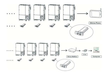
• Through RS232 interface- wireless module-Data logger-Internet.
