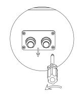
2. Slightly loosen the swivel nut, remove the filler-plug from the M16 cable gland.
