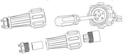
2) Connect 5 cables into their respective channels on the AC terminal, while 'N' represents Neutral, '1, 2, 3' represent 3 line channels and 'E' is ground, tighten all screws (1.0Nm (9 lbf.in.) max).
