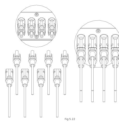
3 Check the assembled DC connectors for correct polarity and connect them to the inverter.
