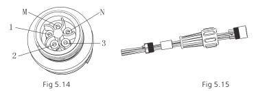
3) Insert the contact into the body with slotted screwdriver (1.13Nm (10 lbf.in.) to 1.36Nm (12 lbf.in.)), screw up other components of the connector.
