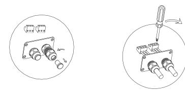
3. Make the cable through the hole of cable gland and put the cable into the RS485 terminals, fix all cables with screwdriver ('1'to'1', '3'to'3', '2' to the shielding layer
