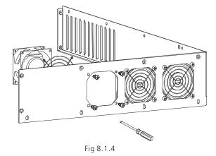
9. After cleaning, assemble the inverter in reverse order. If you cleaning the fans using water please make sure the fans, cables and connectors are dry before assembling.
