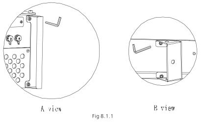
3. Remove the handles on both sides of UE inverter as fig.8.1.1 B View show.
