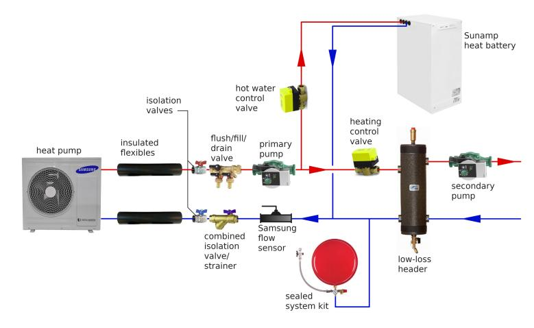
The pipework installation is very like installing a Samsung ASHP with an unvented cylinder as you normally would. The schematic above shows a primary/secondary pumping arrangement with a header but it is also fine to use an automatic bypass valve on the heating pipework if you'd prefer.
