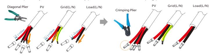
b) Gird(PE) strip the grounding cable insulation(length"L2", insert the stripped cable into the R type terminal, and then clamp it.
