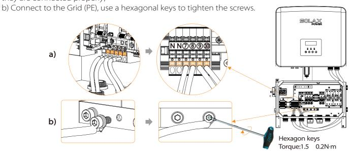
2) PV(PV1+/PV1-/PV2+/PV2-) /Gird(L/N/PE) /Load(L/N) side connection.
