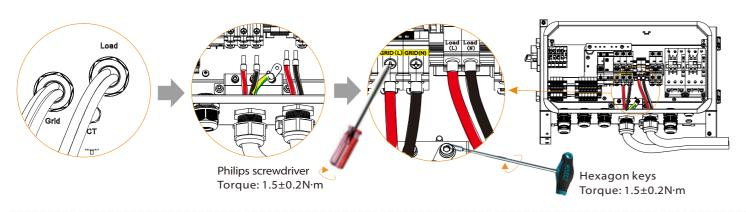
5) Pass the battery power wire through the BAT port of The X1-Matebox, then find the BAT+ and BAT-ports in the X1-Matebox, insert each wire accordingly, and use the philips screwdriver to lock the screws.
