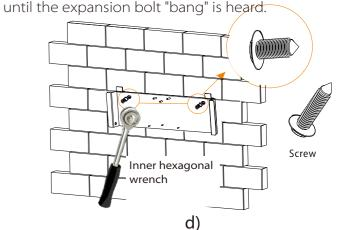
Step 4: Finally install the X1-Hybrid G4 inverter bracket (please refer to the X1-Hybrid G4 inverter quick installation guide).
