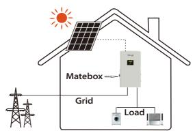
Diagram A: Neutral line and PE line are separated from each other, all loads connect to the Off-grid port;
