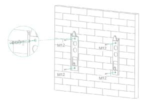
**3.** Mount the All in One onto the mounting bracket. Adjust the height of the supporting feet to ensure the unit is level and attach the securing screws to the brackets, ensuring the weight is on the feet, not the brackets. Brackets are there for stability.
