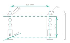
**2.** Fix the mounting bracket to the wall using the expansion bolts. Please note: the brackets are sided.
