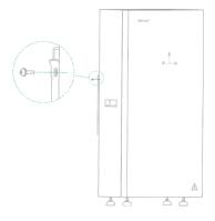
**4.** Re-insert the battery modules into the shelves of the All in One battery compartment. Secure the battery modules using the fixings provided. Re-attach waterproof cover.
