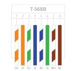
**Please note**: The communication cable must be terminated with a RJ45 plug at either end to connect the All in One to the Giv-Gateway. Ensure the wiring configuration into the RJ45 is the same both ends, a cross-over cable will not work. A standard Ethernet Cat5/6 cable will suffice here wired to T-568B standard if doing locally.
