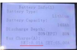
Battery Communication Fail. The battery icon is gone. Please Check battery type and Dip switch.
