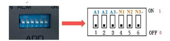
$Dip1^{3}$  to define Master/Slave mode : The Master is binary 0 , the Slave Battery from 1-3
