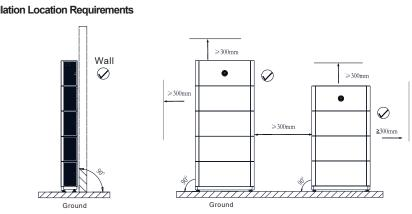
**Note**: When mounted on the ground, a maximum of six battery modules can be stacked. If you are installing more than four modules you are advised to install them in two columns.
