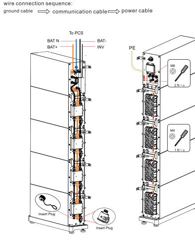
**Note:** It is not recommended to install a DC circuit breaker between the battery system and the PCS. If you want to install a DC circuit breaker with rated working voltage greater than 1000V and rated working current greater than 63A, do not operate the DC circuit breaker with power-on, otherwise the machine may be damaged.
