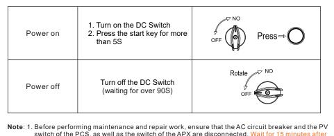
switch of the PCS, as well as the switch of the APX are disconnected. Wait for 15 minutes after off. Do not perform any operations until the system is completely shut down.
