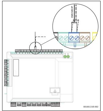
Fig. 17 EMS connection on the installer module
