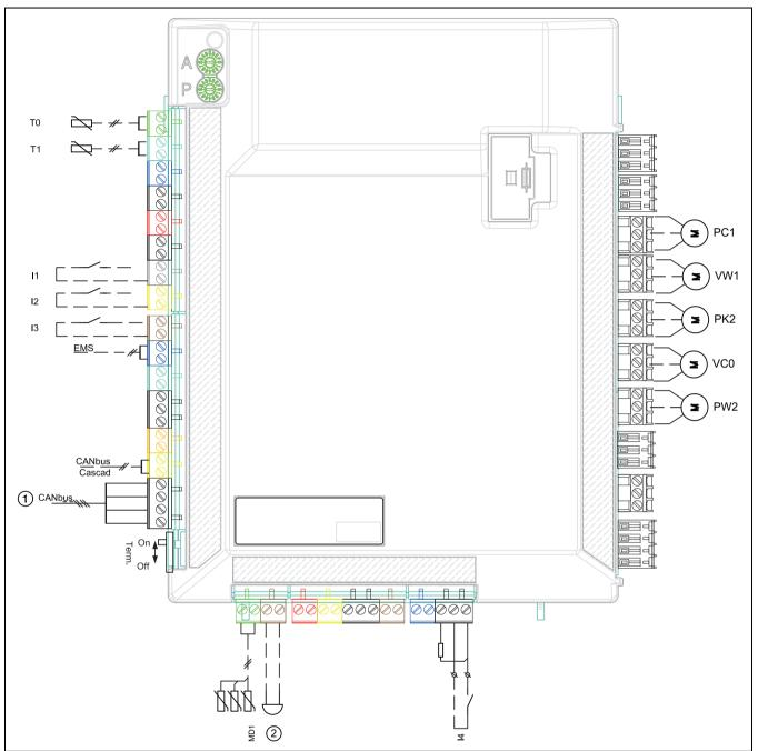
*Fig. 13 Connections to installation module*
