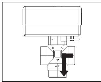
Fig. 20 Contact closed, connection A open
