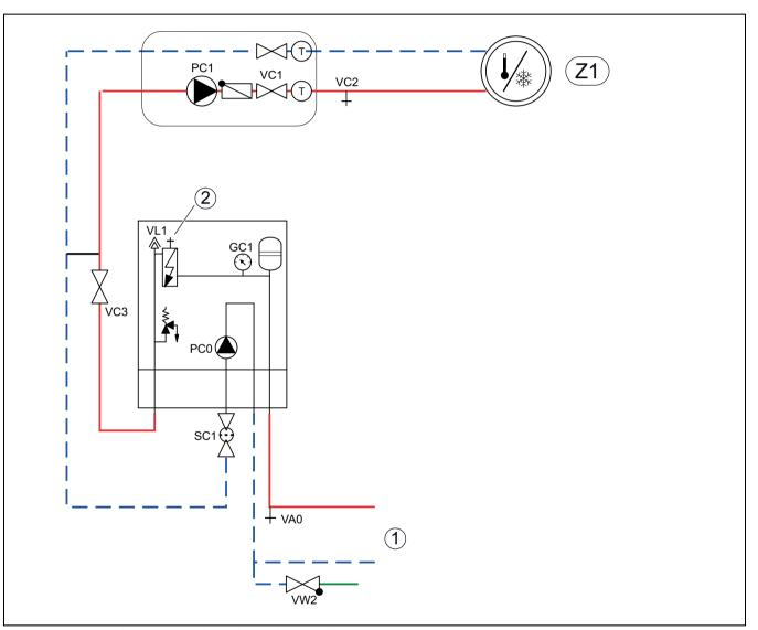
Fig. 15 Indoor unit with an integrated electric booster heater and heating system
