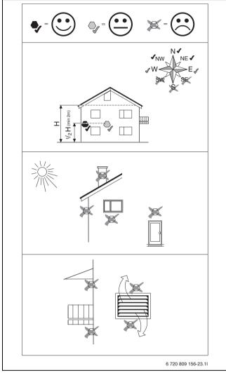
Fig. 9 Position of the outdoor temperature sensor
