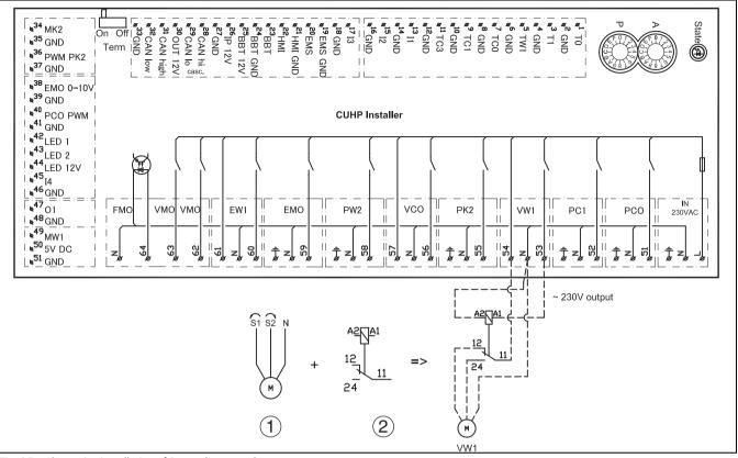
Fig. 35 Alternative installation of 3-way diverter valve
