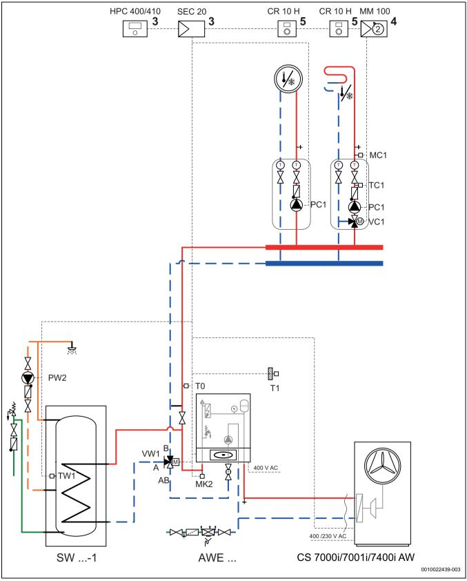
Fig. 29 Electric booster heater with water heater
