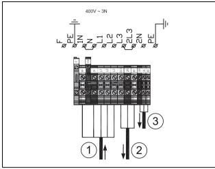
Fig. 11 Electrical standard connection for the integrated electric booster heater
