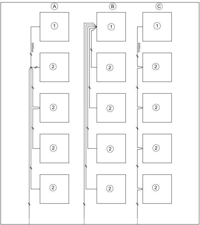
Fig. 14 Connection alternative for EMS bus
