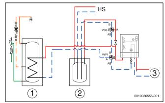
Fig. 25 Buffer, VCO bypass valve
