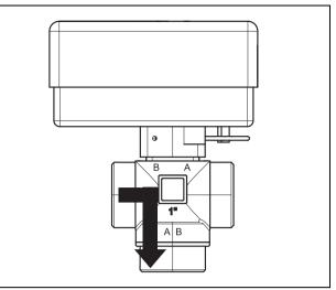
Fig. 21 Contact open, connection B open
