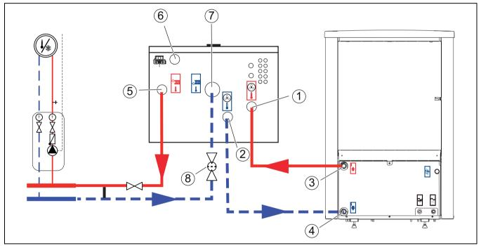
Fig. 6 Connection of the indoor unit with electric booster heater to the heat pump and heating system
