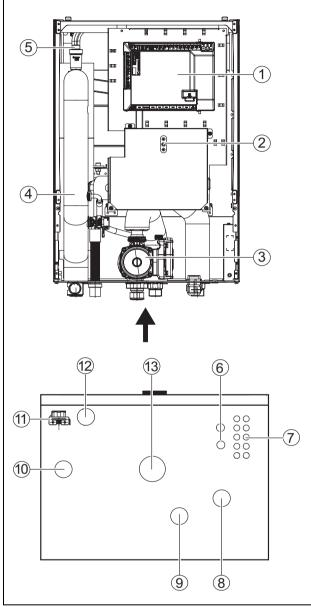
Fig. 3 Components and pipework connections of the indoor unit with auxiliary heater
