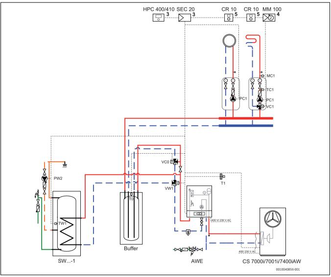
Fig. 30 Electric booster heater with water heater
