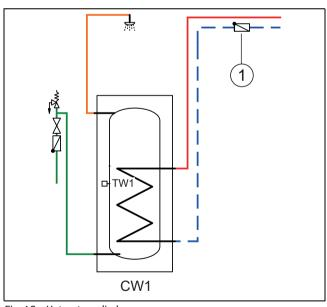
Fig. 18 Hot water cylinder
