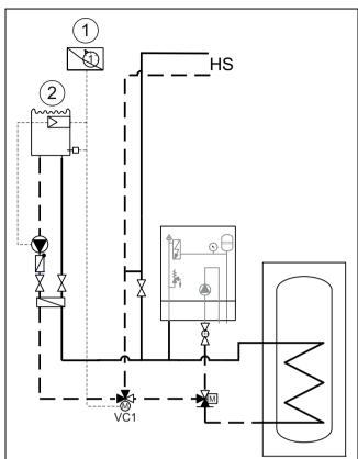
Fig. 24 Example showing swimming pool installation
