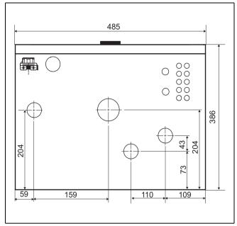
Fig. 5 Dimensions and connections
