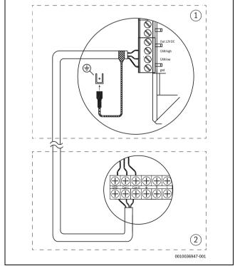
Fig. 20 CAN-BUS connection
