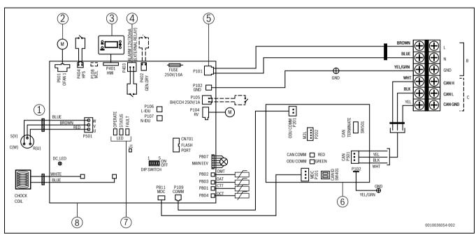
Fig. 26 Wiring diagram outdoor unit single phase CS3400iAWS 4 OR-S
