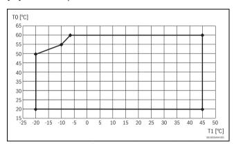
Fig. 24 Operating range of heat pump in heating mode without auxiliary heater
