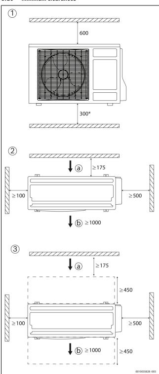
Fig. 4 Minimum clearances (mm)
