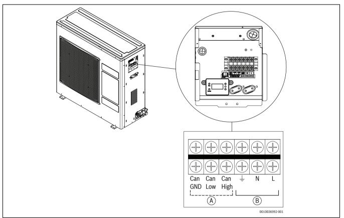
Fig. 19 Cable connections
