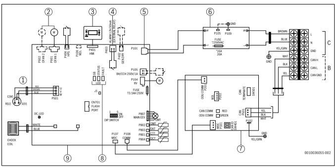
Fig. 27 Wiring diagram outdoor unit single phase CS3400iAWS 6 OR-S, CS3400iAWS 8 OR-Sand CS3400iAWS 10 OR-S
