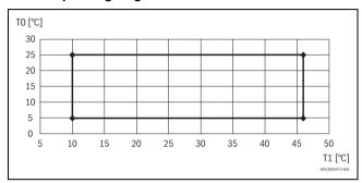
Fig. 23 Operating range of heat pump in cooling mode
