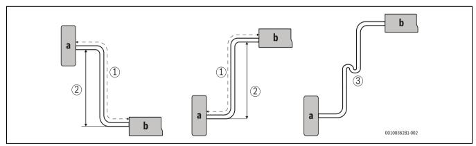
Fig. 10 Pipe length and elevation
