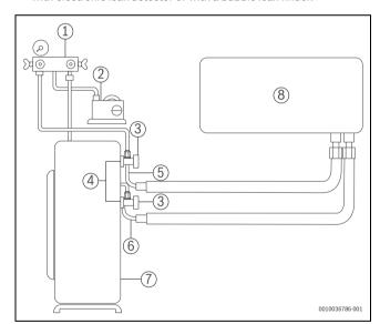
Fig. 18 Vacuum, charging and leakage test
