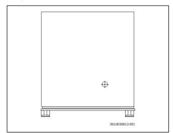
Fig. 5 Package with marked centre of gravity
