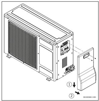
Fig. 14 Remove the side cover
