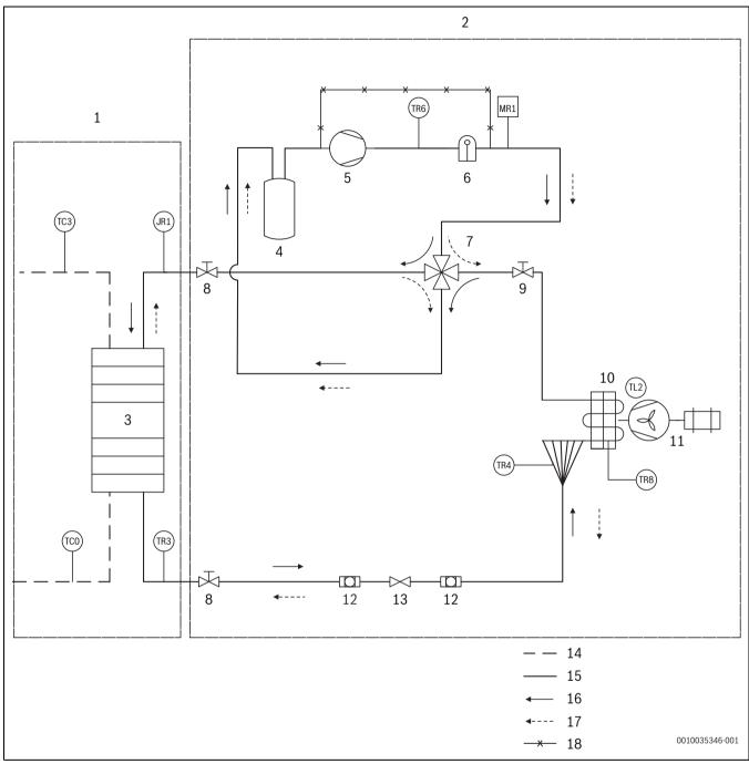
Fig. 25 Diagram of the refrigerant circuit
