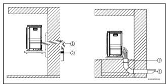
Fig. 17 Connection of the outdoor unit with the indoor unit
