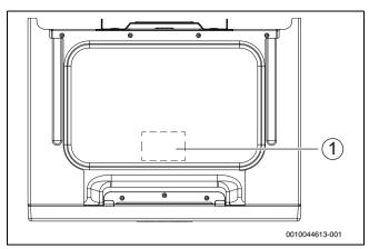
Fig. 7 Type plate position, inside of the appliance
