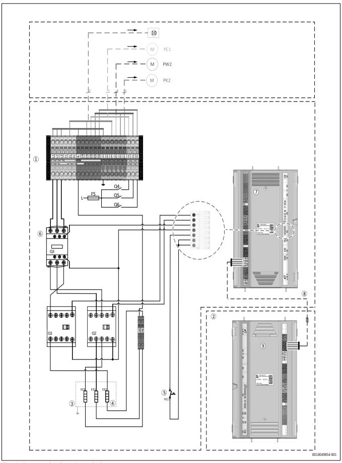
Fig. 41 Power supply indoor unit, standard
