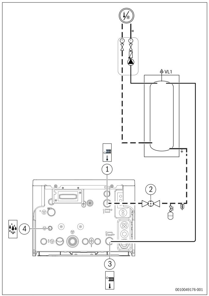
Fig. 17 Connection of the indoor unit to the heating system
