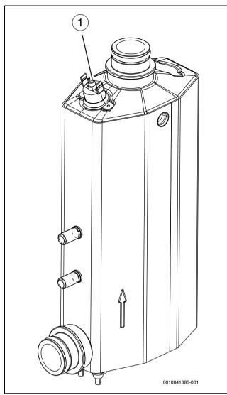
Fig. 35 Electrical heater
