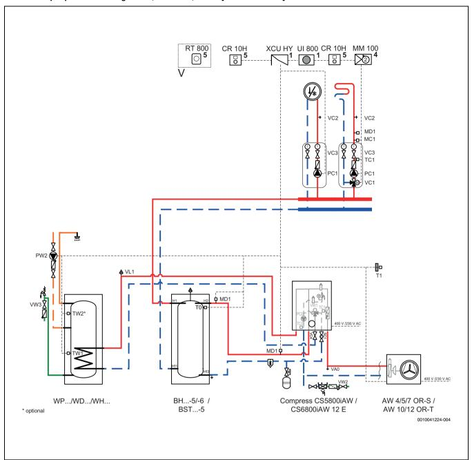
Fig. 38 Heat pump, two heating circuits, indoor unit, buffer cylinder and DHW cylinder
