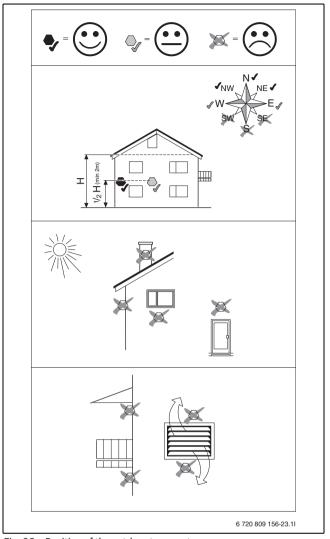
Fig. 23 Position of the outdoor temperature sensor
