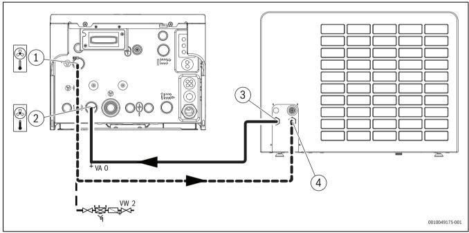
Fig. 16 Connection of the indoor unit to the heat pump
