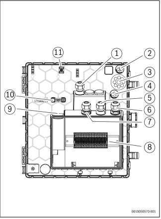
Fig. 27 Cable feeds to electric box
