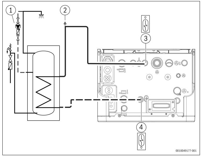
Fig. 18 Indoor unit connections tap water
