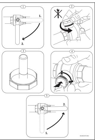
Fig. 36 Cleaning the strainer
