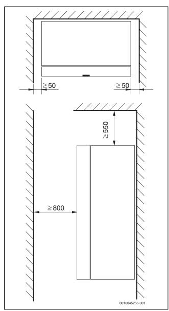
Fig. 4 Minimum clearances to surrounding walls or parts (mm)
