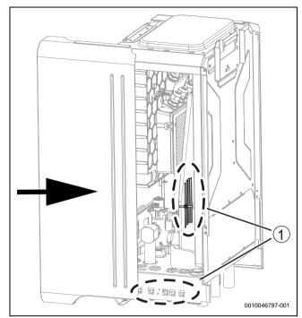
Fig. 29 Slide the side cover in place
