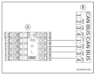
Fig. 20 CAN-BUS heat pump - indoor unit
