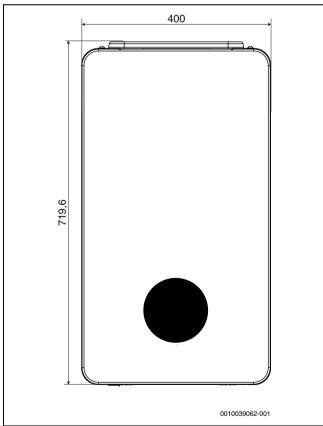
Fig. 2 Dimensions front view (mm)
