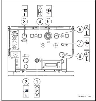
Fig. 6 Pipework connections
