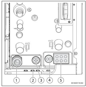
Fig. 25 Cable inlets to the indoor unit
