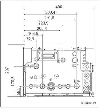
Fig. 3 Dimensions connections, bottom view (mm)
