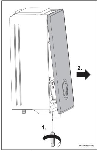
Fig. 10 Remove the front
