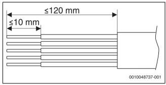
Fig. 24 Wire striping mains feed connection
