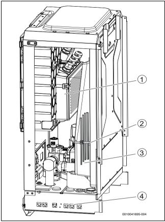
Fig. 26 Cable routing
