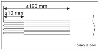
Fig. 21 Wire striping CAN-BUS
