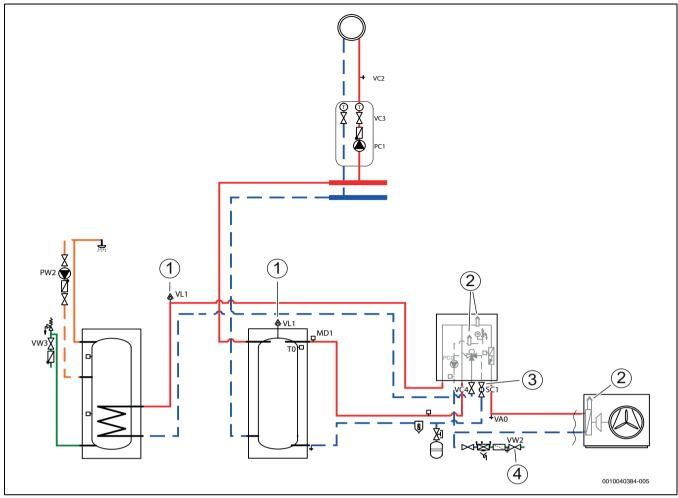
Fig. 19 Indoor unit, heat pump, DHW cylinder and heating system with buffer
