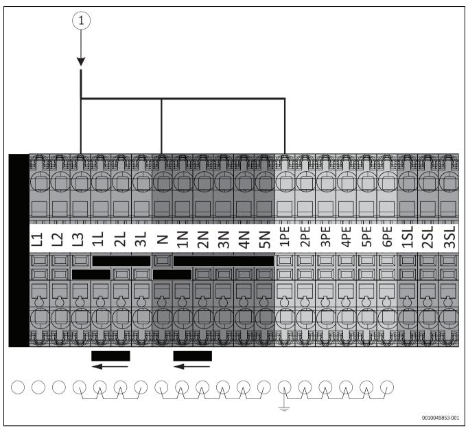
Fig. 31 Electrical connection for single-phase, 3kW only
