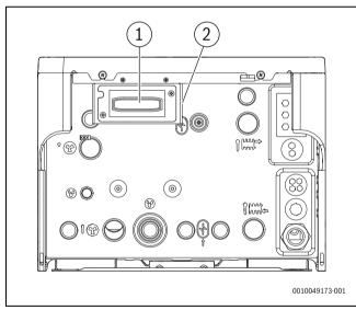
Fig. 9 Connect-Key K30RF placement
