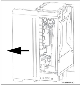
Fig. 13 Remove the side cover
