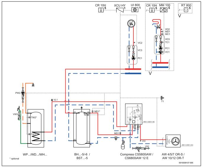
Fig. 37 Heat pump, indoor unit, buffer cylinder and water heater
