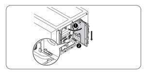
4 Insert the cables at the rear of the unit, and route them through the factory mounted cable sleeves into the switch box.
