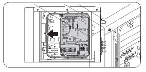
**3** If the plate is rotated to where the hook is, it will be fixed to the hook.
