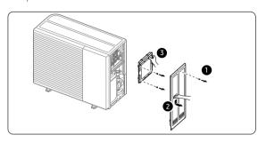
2 Remove 2 screws and pull the plate to the left.
