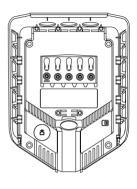
**Backplate**For attaching and connecting to the charging infrastructure.
