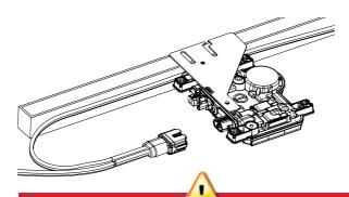
WARNING: Install sealing caps on all unused AC connectors as these connectors become live when the system is energised. aling caps are required for protection against moisture ingress
