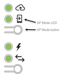
2. The AP Mode LED  $^{\bullet}$  remains solid green when AP mode is enabled and active. AP mode times out after eight hours. This LED is usually off during normal Envoy-S operation.
