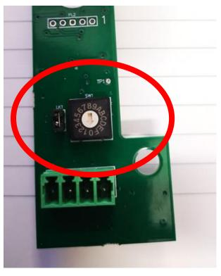
Figure 1 - Rotary switch to select Maximum current rating
