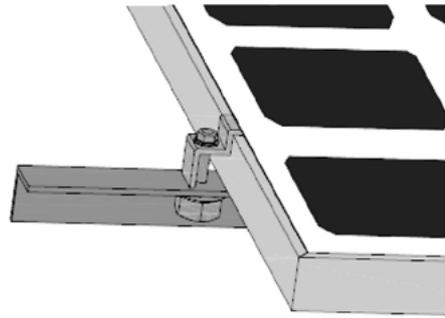
**Clamp Mounting on Long Sides of the Frames**
