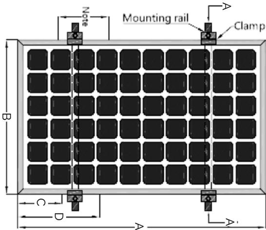
**Clamp Mounting on Short Sides of the Frames**
