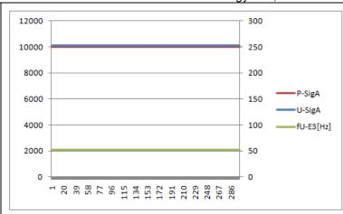
**2.Power Quality – Harmonics:** These tests should be carried out as specified in BS EN 61000-3-2. The chosen test should be undertaken with a fixed source of energy at two power levels a) between 45 and 55% and b) at 100% of Registered Capacity. The test requirements are specified in Annex A1 A.1.3.1 (Inverter connected) or Annex A2 A.2.3.1 (Synchronous).
