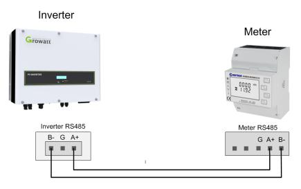
Inverter and meter connection 1 (750-3000-S, 2500-5500MTL-S, 3-15KTL3-S)
