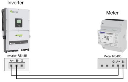
Inverter and meter connection (17-25KTL3-S, 30-50KTL3-S)
