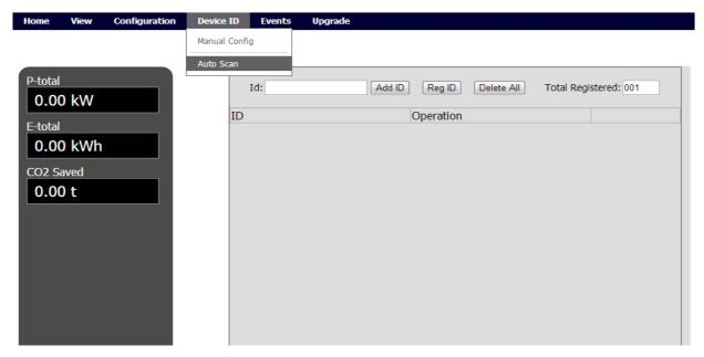
Click "Scan ID" to start automatic search for microinverters. When the DTU detects all the microinverters' IDs, you need to click "Reg ID" to finish registration. If the DTU cannot detect all the microinverters in the system over 30 minutes, please use manual mode instead.
