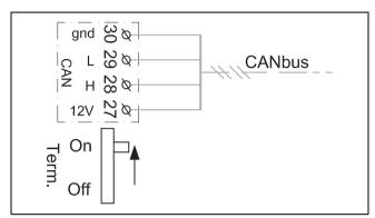
Fig. 18 Termination CAN-BUS
