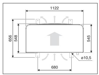
Fig. 6 Dimensions of heat pump models 13 OR-S/T-17 OR-T, view from top
