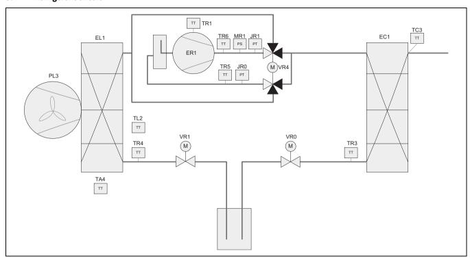
Fig. 23 Refrigerant circuit
