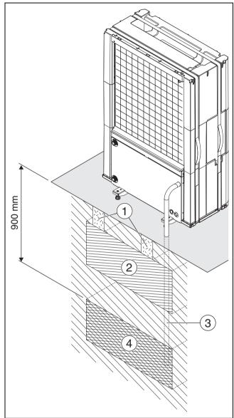
Fig. 11 Condensate pipe in gravel bed
