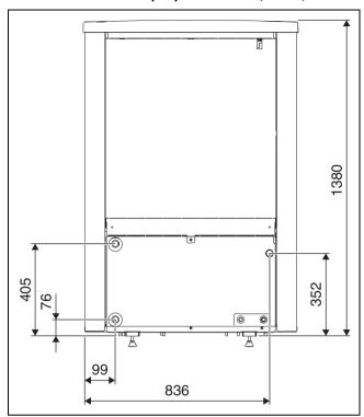
Fig. 3 Dimensions and connections of heat pump models 5 OR-S-9 OR-S
