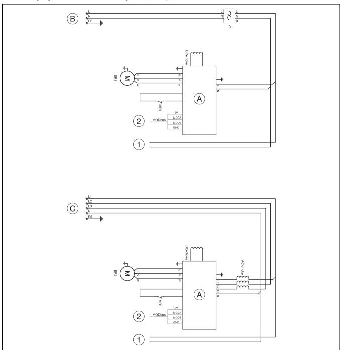
Fig. 24 Wiring diagram for transformer, alternating current / three-phase current
