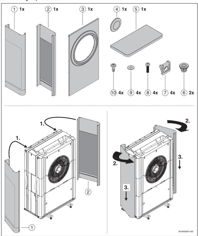
Fig. 20 Installing side panels and cover
