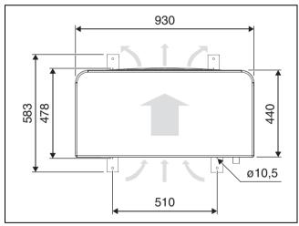
Fig. 4 Dimensions of heat pump models 5 OR-S-9 OR-S, view from top
