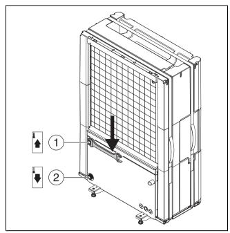
Fig. 17 Connections of heat carrying medium pipes, valid for all sizes
