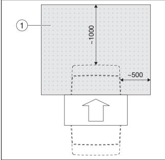
Fig. 10 Danger! Ice formation in front of heat pumps with noiseattenuating device (accessory)
