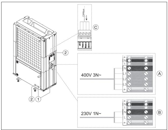
Fig. 19 Cable conduits and control device
