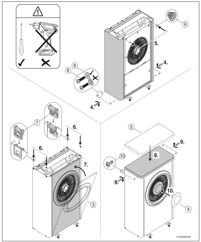
Fig. 21 Installing side panels and cover
