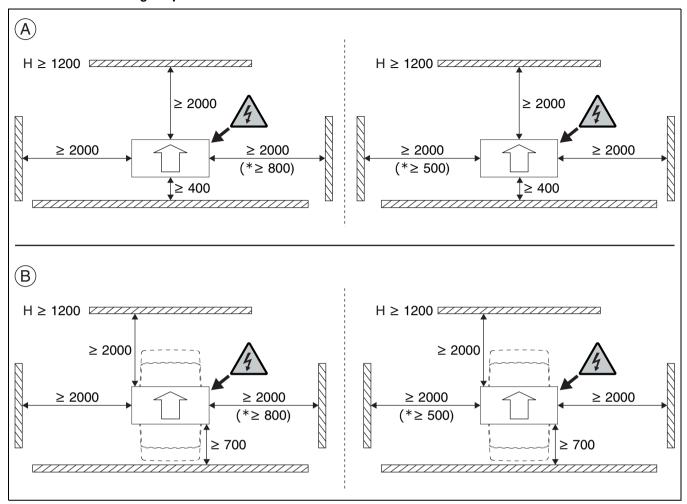
Fig. 7 Clearances during setup
