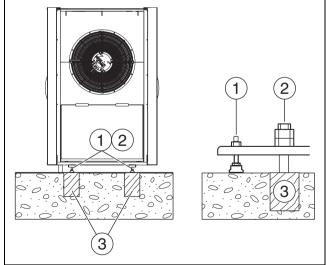
Fig. 13 Fastening the heat pump
