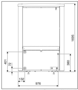
Fig. 5 Dimensions and connections of heat pump models 13 OR-S/T-17 OR-T
