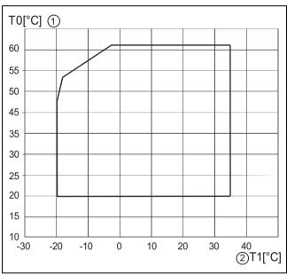
Fig. 22 Heat pump without auxiliary heater
