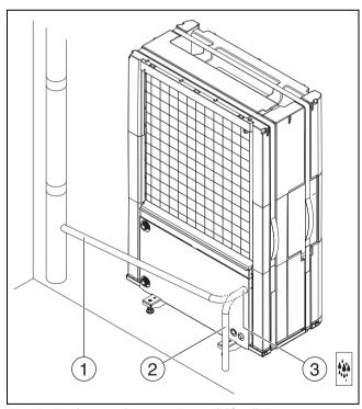
Fig. 16 Condensate tube connections, valid for all sizes
