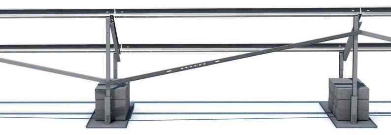
Piled and X-Anchor Systems Piled and X-Anchor systems with less than 4 bays only require one pair of braces, in an 'x'
