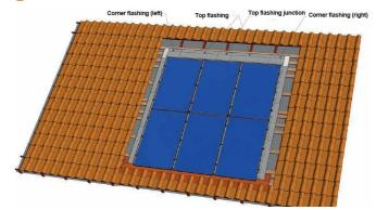
Position the attach angles and the top flashings so that it fits the module thickness. Make cuts on the attach angle at the position of the GSE panel corrugations.
