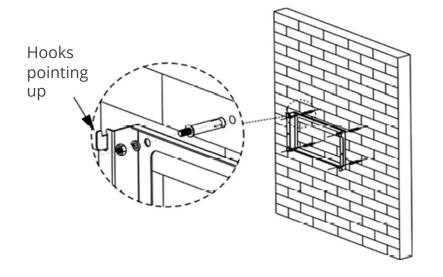
Brackets should be installed with the hooks pointing upwards and secured using the 4 fixings points provided.
