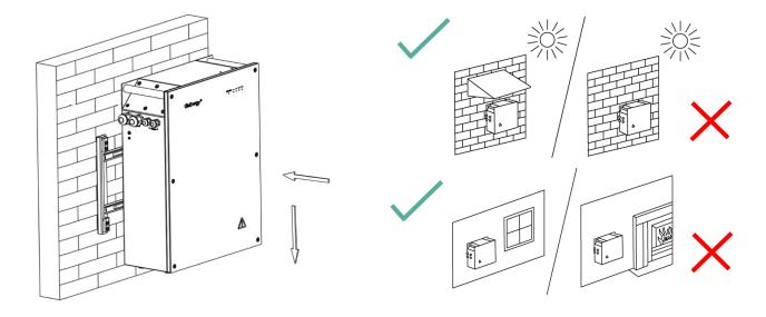
All batteries must be secured to the wall using the fixings provided, even if the weight of the battery is on the floor.
