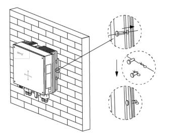
Once the inverter is securely mounted onto the bracket, the locking pin should be installed on both sides.
