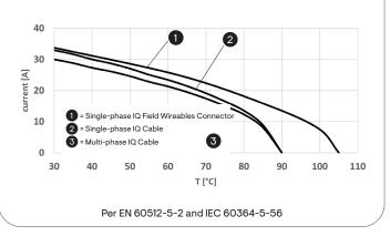
Note: It is recommended to increase the ambient temperature by 20°C to account for solar radiation and under-module heating impact on IQ Cable temperature.
