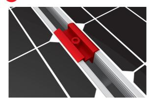
Use two universal module middle clamp OneMid between two modules. Klick the Stance in the notches. Place clamps on the module frames and fix them. Tightening torque 14 Nm.
