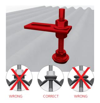
Before mounting the solar fasteners, remove any burr from the surface of the profile sheets. Insert the Hangerbolt into the pre-drilled hole and screw in.
