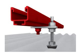
Ensure correct position of T-bolt. After inserting into the lower chamber of the rail, the T-bolt is turned 90 degrees counterclockwise. Lock the projected K2 module carrier rail Solid on the adapter plate with an M10 T-bolt and self-locking nut. Tightening torque: 32 Nm
