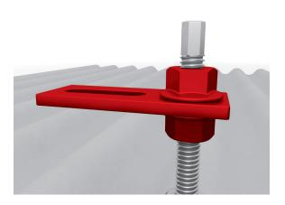
Screw the locking nut under the adapter plate into the correct position to define the height of the adapter plate. After correct adjustment of the adapter plate, fasten the upper locking nut.
