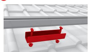
Lay Mounting Rail on joint with rail connector and connect with T bolts and self-locking nuts. The rail joint may not be in the range of the roof fastener. Tightening torque 16 Nm.
