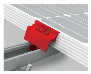
Fix the module in place at the end of a row with universal module end clamp OneEnd. Klick the Stance in the notches. Alternatively use the standard end clamp. Insert the MK2 nut into the mounting rail and turn clockwise by 90°. Place clamps on the module frames and fix them. Never mount module end clamps directly on the rail joint or end of the rail! (Spacing: min. 50 mm from edge of module frame). Pay attention to the mounting instructions by module manufacturer!
