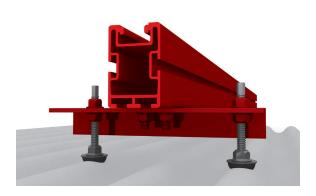
The K2 Bridge is mounted on two Hangerbolt instead of the adapter plate in order to achieve greater span widths. Depending on type, the rail is fixed to the Bridge with one or two M10x30 T-bolts.
