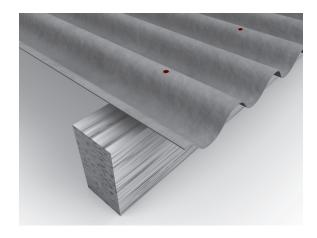
Measure the screw distances according to statics or K2 Base. Check position of purlins and pre-drill through the fibre cement profiles into the purlins.
