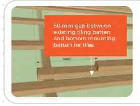
C: 50mm gap between existing & mounting batten
