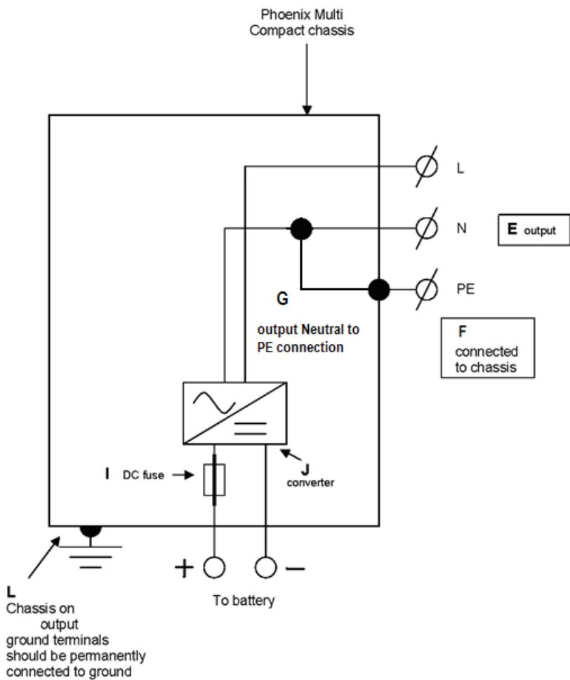
This ground wire "G" connects the output neutral to ground. It must be cut/removed if a floating output is required or reposition to "dummy" terminal.
