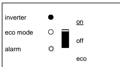
The inverter is switched on and supplies power to the load.
