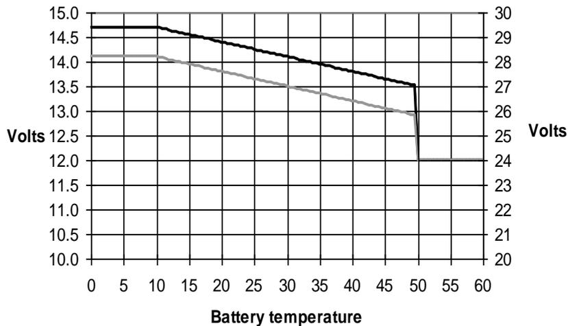
**EN** Default output voltages for Float and Absorption are at 25 °C.
