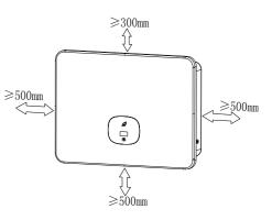
Fig 5.2 Installation dimensions for one inverter
