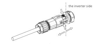
Fig 6.11 2. Insert the H-shaped tool and pull it out of the socket.
