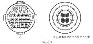
$1.Strip the cable 10 \mbox{mm} through the waterproof gland, thread sleeve, and tighten the screws.$
