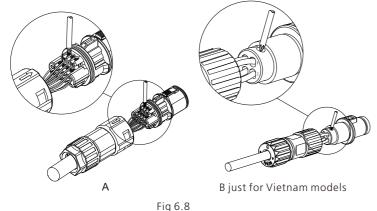
2.Push the threaded sleeve into the socket and tighten the waterproof gland.
