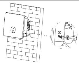
Fig 6.1 Grounding diagram
