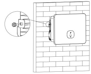
Fig 5.9 Schematic diagram of inverter wall mounting
