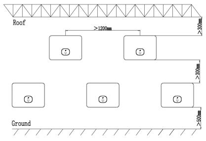
Fig 5.3 Installation dimensions for multiple inverters
