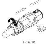
Remove the signal connector 1.Press down the fastener and pull it out of the inverter.
