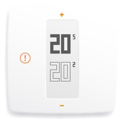
In this case, the Thermostat communicates with the server every 10 minutes to get the latest changes to the schedule or the manual setpoints.
