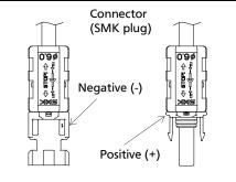
Figure 3: Configuration of Junction Box
