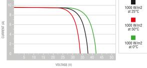
\*STC: (Standard Test Condition) Irradiance 1000W/m²; Module Temperature 25°C; Air Mass 1.5 \*\*NOCT: (Nominal Operation Cell Temperature) Sun 800W/m²; Air 20°C; Wind speed 1m/s \*\*\*Pallets can be stacked up to two
