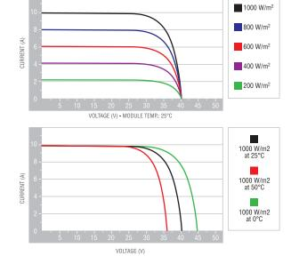
\*STC: (Standard Test Condition) Irradiance 1000W/m²; Module Temperature 25°C; Air Mass 1.5
