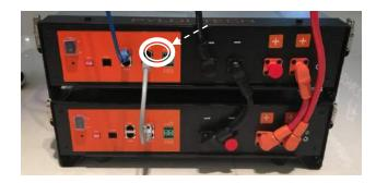
(3) Touch the **start button** of **master battery** to power on, all the battery LED light will be on one by one from the Master battery:
