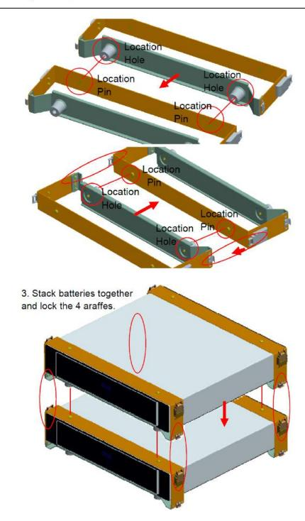
Aim at the 4 pare of Location Pin and Location Hole, stack the batteries together. And hasp the 4 agraffes together.
