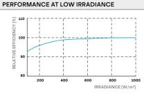
Typical module performance under low irradiance conditions in comparison to STC conditions (25  $^{\circ}\text{C},$  1000 W/m²).
