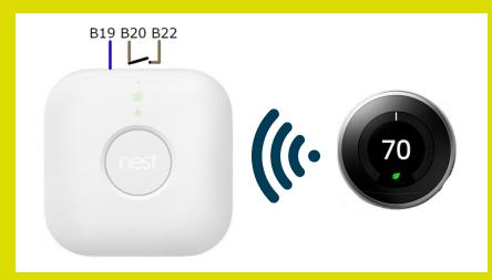
Then set the heat pump to use it as the signal to heat or not by setting FSV 2091 - External Thermostat Application #1 (Floor) to
