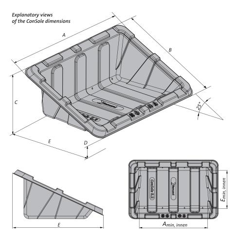
Recommended measurement of ConSole/PV module
