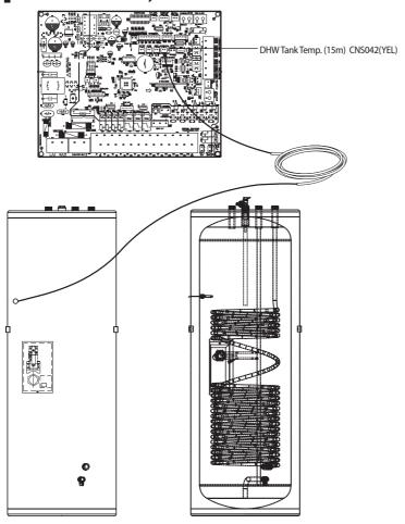
\* Use a correct sensor pocket which is fit for the DHW tank sensor(OD Ø6).
