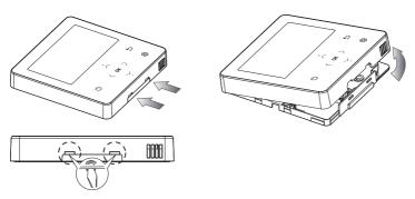
2. Arrange the power cable and the communication cable so that they fit in the housing along the edges of the rear cover.
