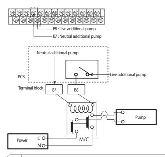
• Terminal of this product is for additional water pump and the maximum allowable current is 0.5 A.
