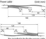
Pre-installed tube for the power cable
