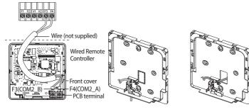
\* Do not tighten the screws on the PCB terminal with excessive force.
