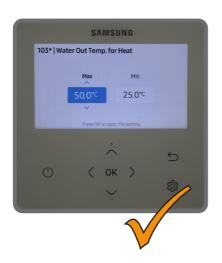
Ensure that the maximum flow temperature has been specified correctly: no more than 55°C for radiators, no more than 45°C for underfloor heating.
