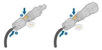
4. Push the insert into the sleeve and tighten the cable gland (torque 2 N·m).
