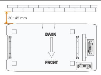
step 5 Place each battery module on top of the base.
