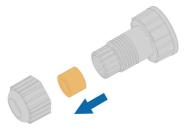
step 3 Insert the RJ45 plug into the front plug connector until there is an audible click, and install the rubber gasket.
