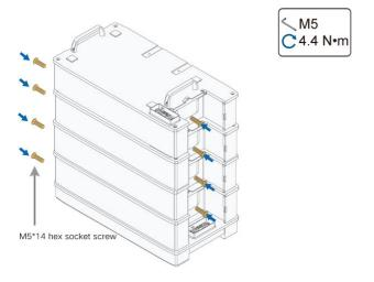
step 8 Connect the switch gear to the base.
