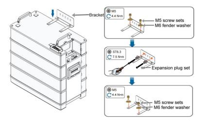
The bracket is mounted on the top battery module.
