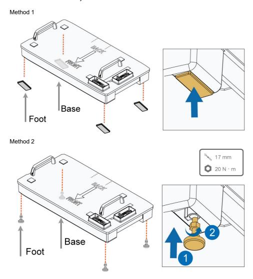
step 2 Align the base with the wall, and keep a distance of 30 mm to 45 mm between the base and the wall. Mark the hole positions of the mounting bracket with a marker according to the required layout of holes.
