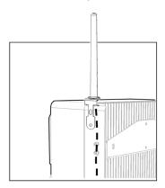
Clip the antenna to a bracket (not supplied by SolarEdge) attached to a vertical surface. SolarEdge recommends using a bracket with the following dimensions:
