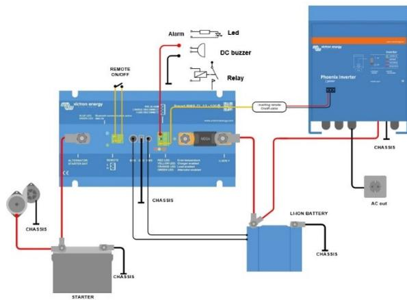
Figure 3: Application example with a Phoenix VE.Bus Inverter rated at 3kVA and more
